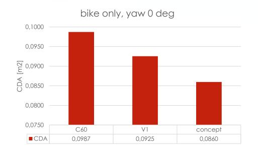
Bikes only (no rider) were tested also. Even if this test is not so useful, due to the huge impact the body of the rider has on the overall aerodynamic of the bike, it's clear the sleek design of the Concept helps to reduce drag considerably.
